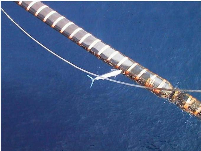
*Here you can clearly see the marlin imbedded in the floating load-hose on the FPSO Girassol. Load operations were shut down for a few days while they replaced the hose. This loading hose is approx 24 inches in diameter, through which the terminal pumps about 250,000 barrels of oil a day. Image courtesy of **Dave Hart**.*
