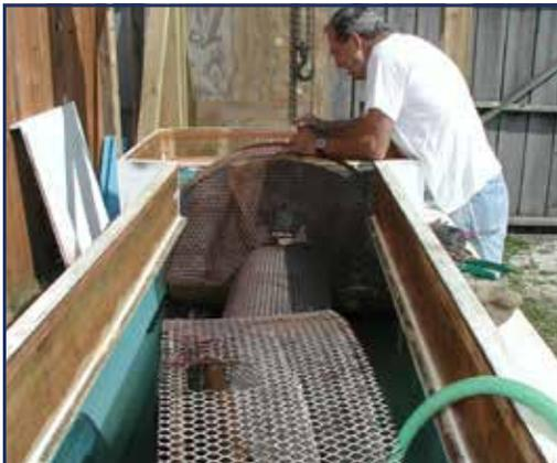
*Paul Adams adjusting custom-fitting anode around screwpile in the electrolysis tank, 2002. (CMM Photo by Rob Hurry)*
